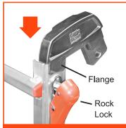
Unlock the Rock Lock. Insert the trestle bracket with the flange on the outside of the rail.
