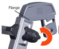
Unlock the Rapid Locks. Insert the trestle bracket with the flange on the outside of the rail.
