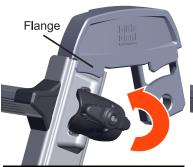
Unlock the Rapid Locks. Insert the trestle bracket with the flange on the outside of the rail.
